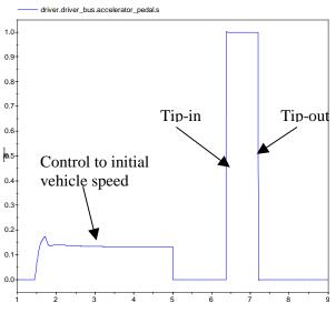
Figure 8: Accelerator pedal profiles
