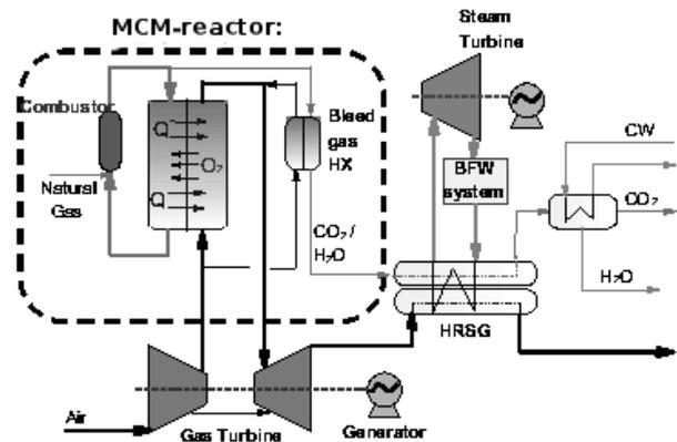
Figure 3: AZEP process flow sheet, inside the dashed square is the reactor system. (from [2])
