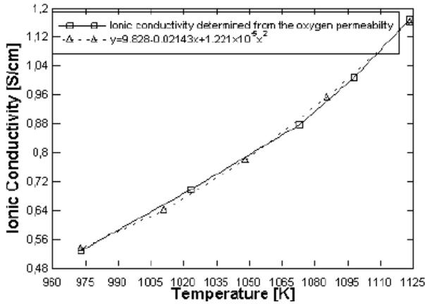
Figure 6: Oxygen ionic conductivity at different temperatures, from [8].
