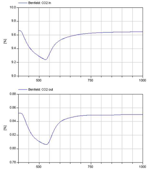
Figure 8: Mole fraction of CO<sub>2</sub> into and out of the Benfield plant section.
