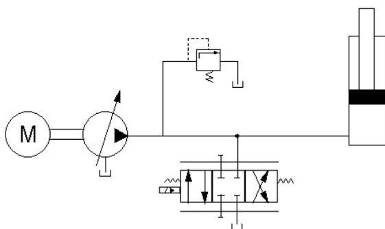
**Figure 2:** Hydraulic circuit of the testing machine
