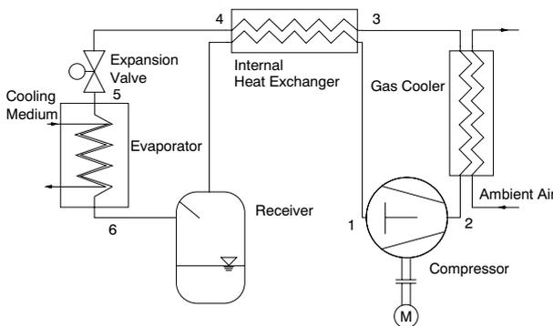
Figure 2: Schematic diagram of a CO<sub>2</sub>-Refrigeration cycle
