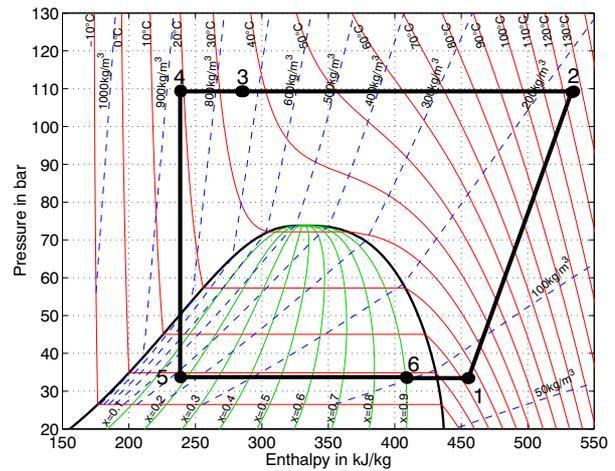
Figure 3: *p,h*-Diagram with states of a CO<sub>2</sub>-Refrigeration cycle
