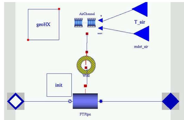
Figure 9: Graphical representation of the heat exchanger model
