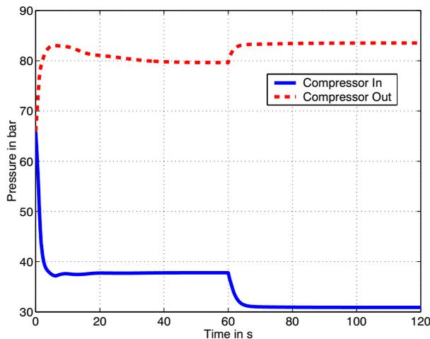
Figure 12: Pressure run at compressor in- and outlet
