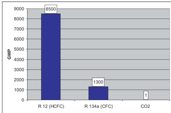
Figure 1: GWP of three different kind of refrigerants; GWP is standardised to 1 for CO<sub>2</sub>
