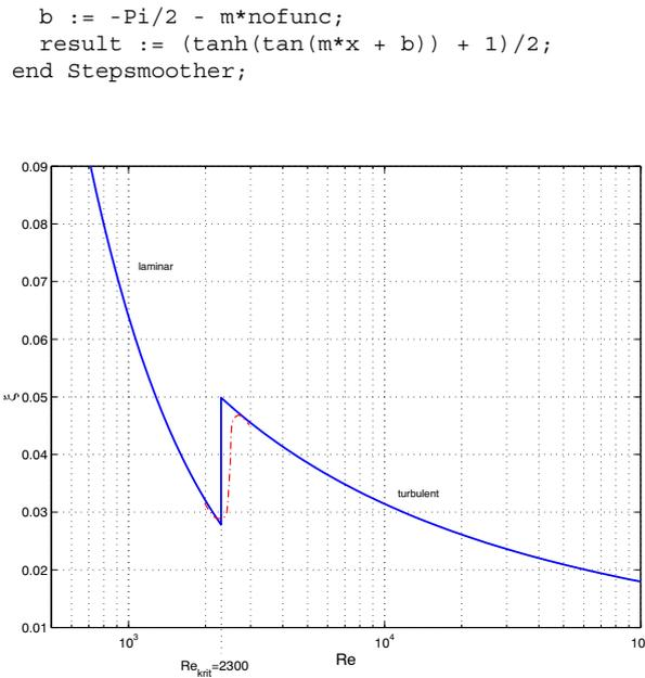
Figure 10: Example for the unsteady transition of the pressure drop coefficient (solid line) and the implemented interpolation function (dashed line)
