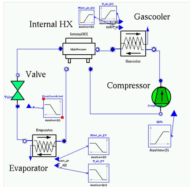
Figure 11: Object diagram of simulated CO<sub>2</sub>-Cycle
