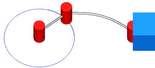
Figure 12: Slider-crank mechanism
