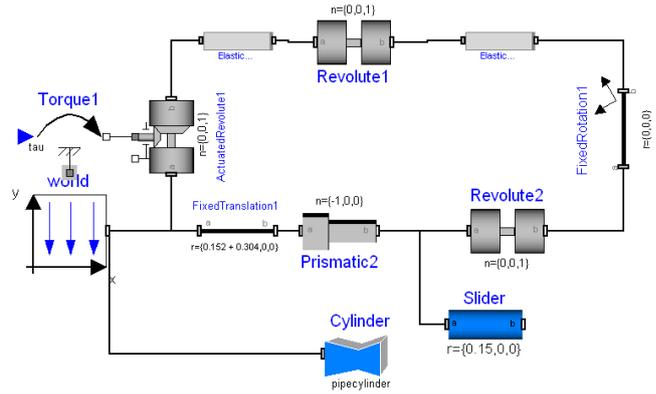
Figure 11: Slider-crank mechanism (Dymola scheme)
