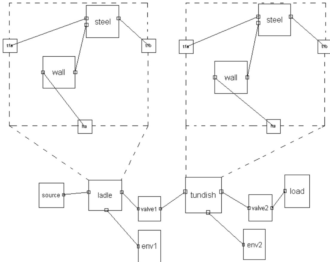
Figure 3: The test structure for the ladle-tundish tandem
