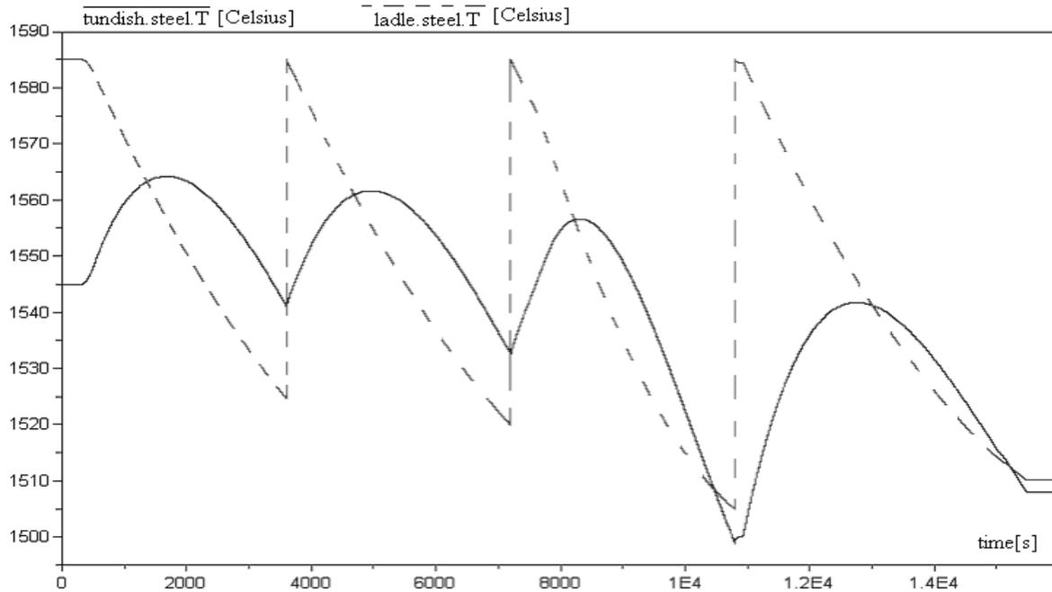
Figure 5: Temperature evolution of the steel in ladle and tundish
