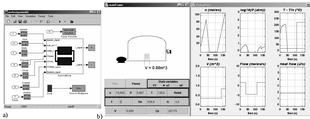
Figure 3: Perfect-gas virtual-lab: a) Simulink model; b) View
