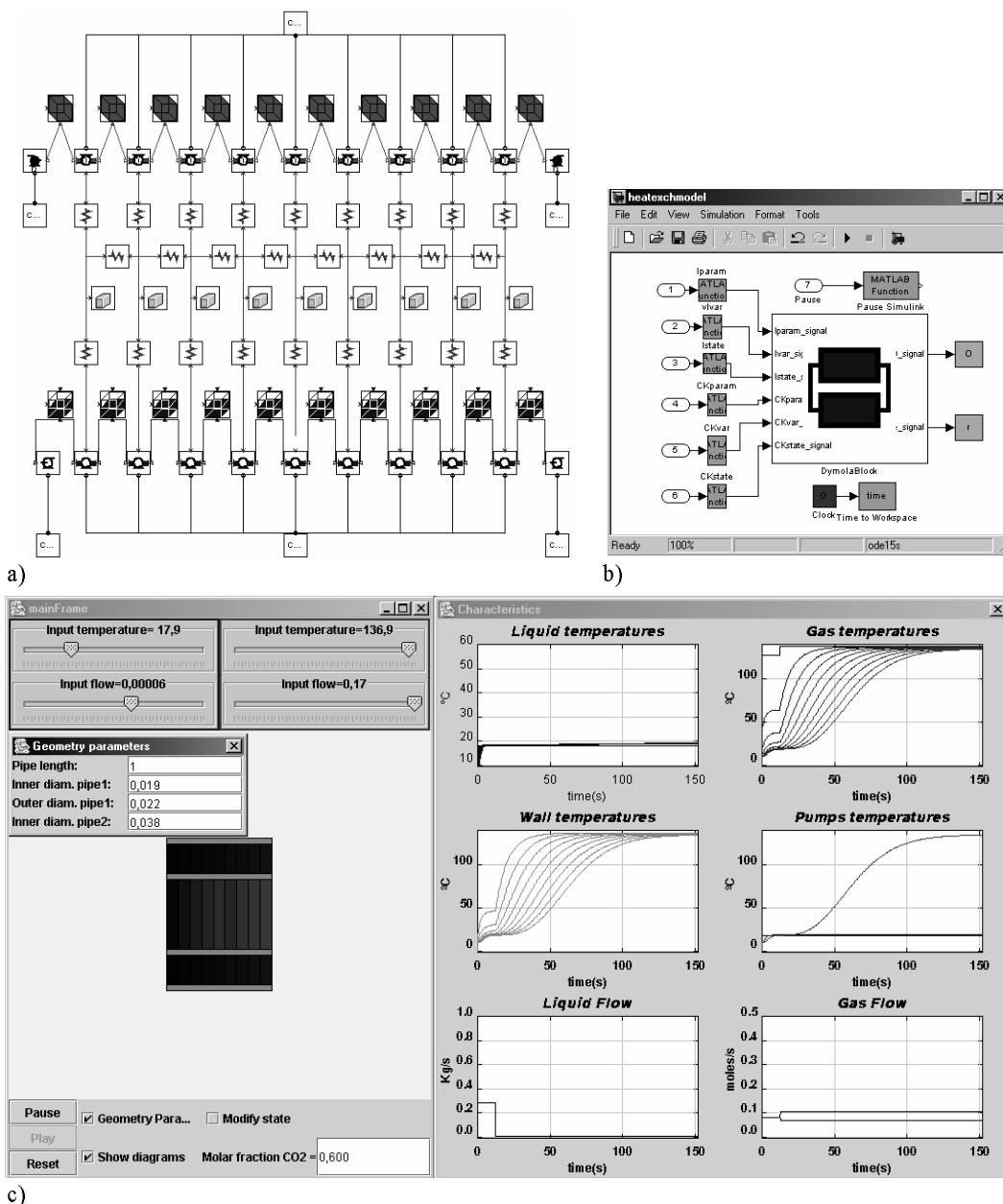
Figure 4: Heat exchanger virtual-lab: a) Physical model; b) Simulink model; c) View
