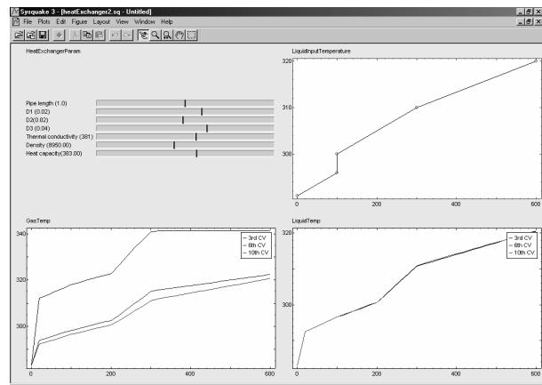
Figure 9: View of the heat exchanger virtual-lab
