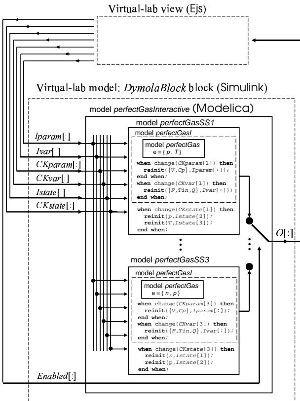
Figure 2: Schematic description of the perfect-gas virtual-lab
