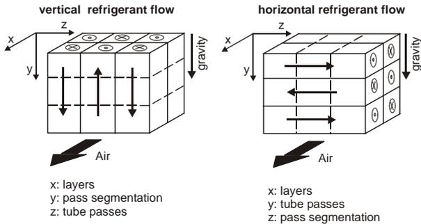
Fig. 3.3: Orientation of component triple in 3D-space
