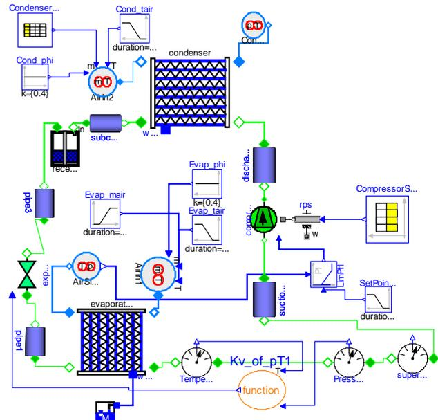
Fig. 4.3: Object diagram of complete R134a refrigeration cycle
