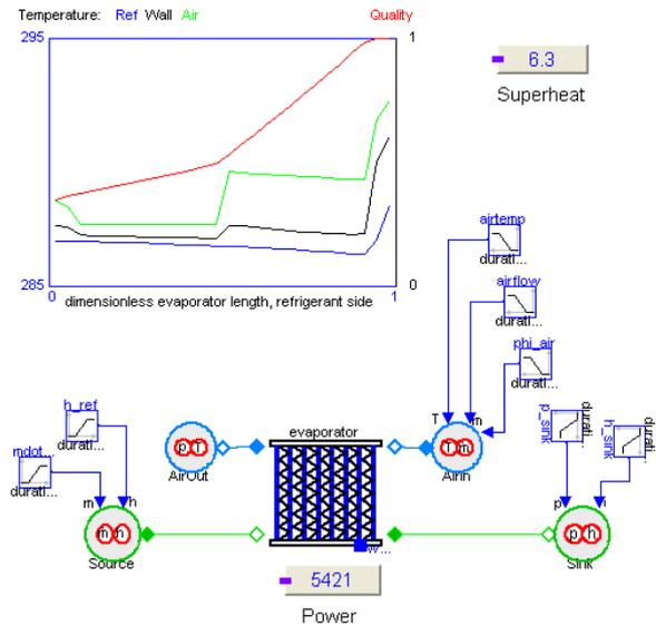
Fig. 3.5: Object diagram of test configuration
