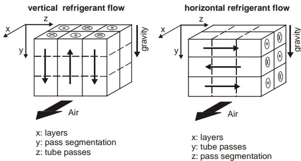
Fig. 3.3: Orientation of component triple in 3D-space
