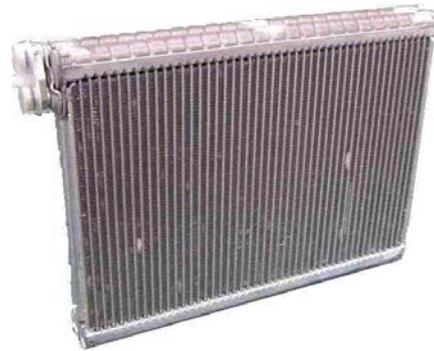
Fig.3.4: R134a-Evaporator, cross counter flow
