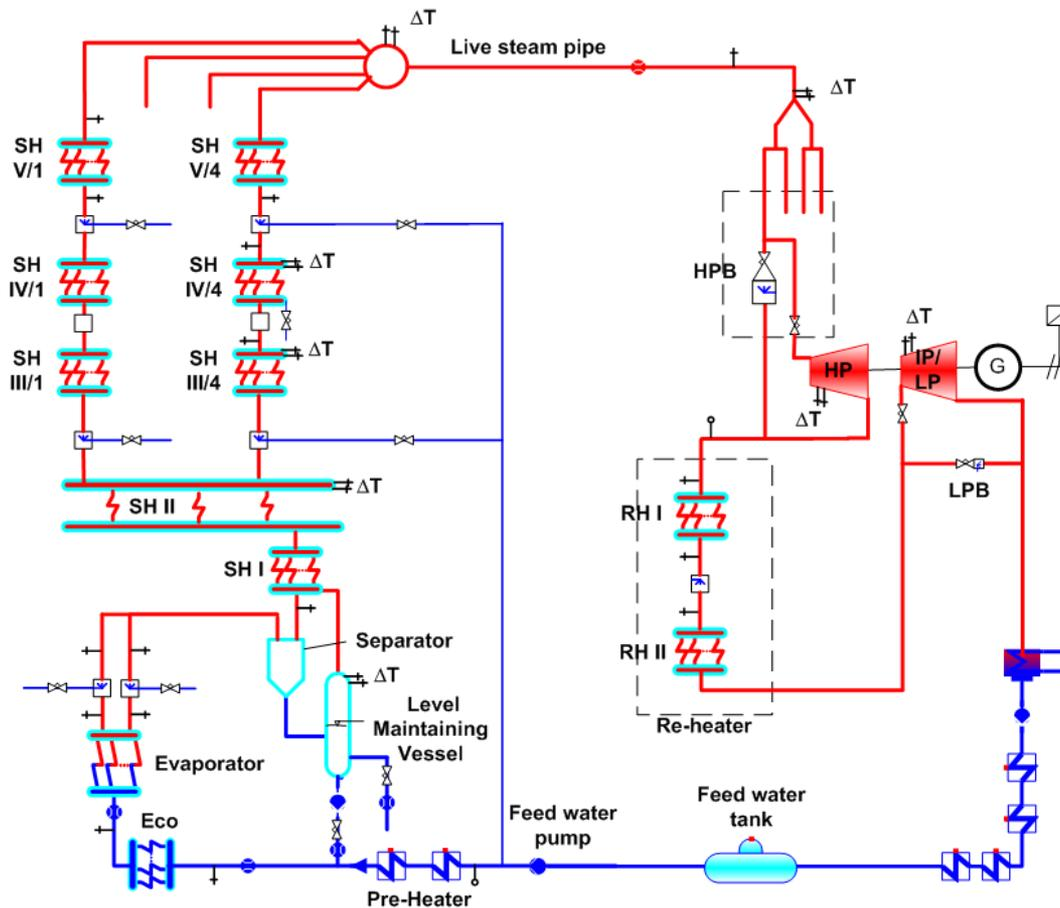
Figure 3: Simplified process diagram of a power plant.
