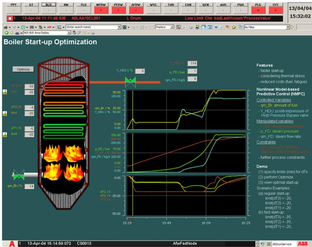
Figure 6: Operator display showing the optimal start-up predicted by the NMPC, in addition to current process values and history logs.
