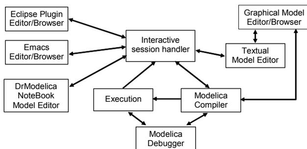
**Figure 2.** The architecture of the OpenModelica environment.
