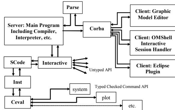
**Figure 3.** The client-server architecture of the OpenModelica environment.
