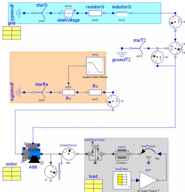
Figure 5: Chipper drive with slip ring motor
