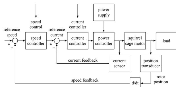
Figure 1: General diagram of a speed controlled drive
