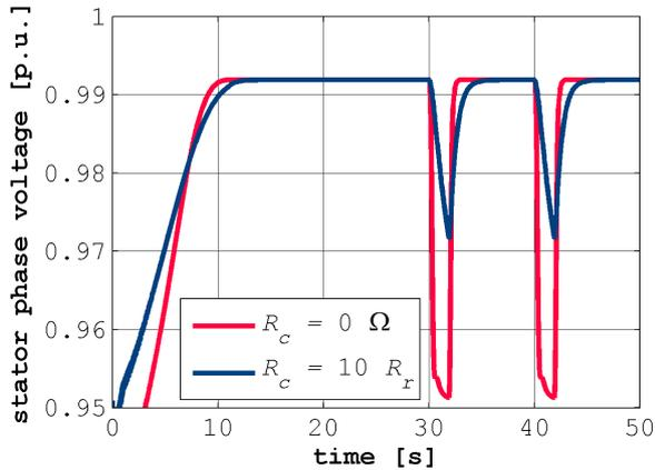
Figure 10: Stator phase voltage during start-up and during periodic loading of the chipper drive with slip ring motor ( $R_c = 0 \Omega$  versus  $R_c = 10R_r$  and  $R_{v,max} = 40R_r$ )
