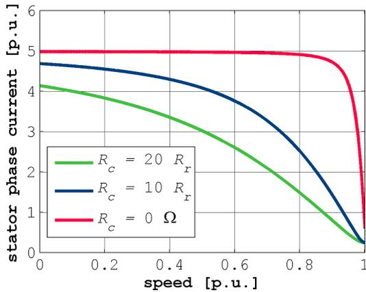
Figure 4: Stationary current versus speed characteristic of a slip ring motor with external rotor resistance
