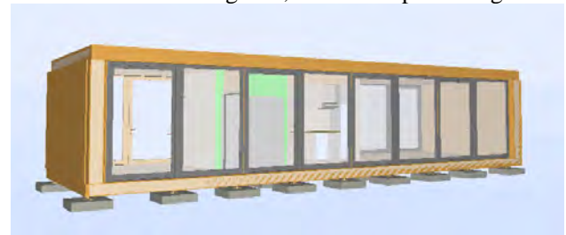
Figure 3. BIM model of the Rooftop building.
