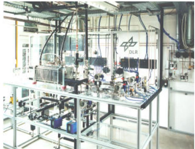
Fig.1: Membrane Fuel Cell Test Facility PEMA at DLR Institute of Technical Thermodynamics
