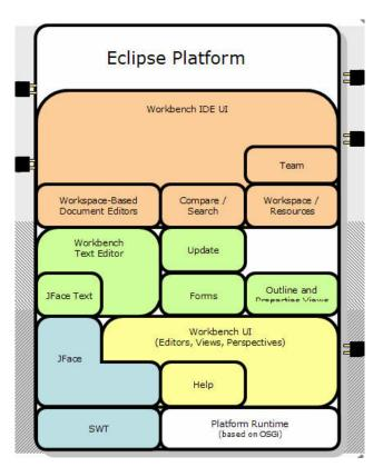
Fig. 1. The architecture of Eclipse, with possible plugin positions marked.
