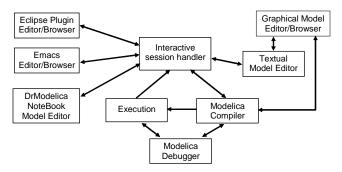
Fig. 2. Architecture of OpenModelica environment.
